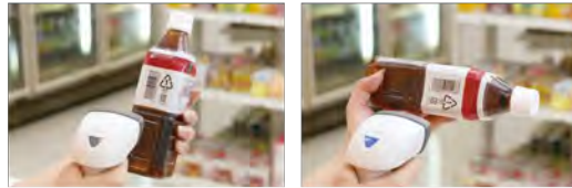
Barcodes can be scanned from any direction. Both horizontal and vertical scanning are possible.
